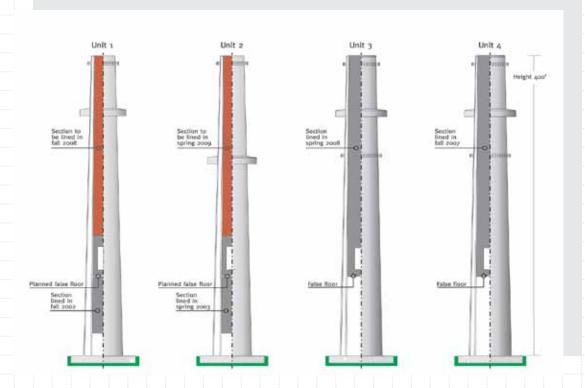
The similar Unit 3 chimney was the second chimney to be lined and was successfully completed as well, in a 6-week outage, during the first quarter of 2008. The applications in the Unit 1 and Unit 2 chimneys are scheduled in the third quarter of 2008 and the first quarter of 2009. The combined surface area of all chimney flues to be lined is 87,445 ft<sup>2</sup>.
