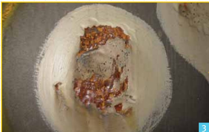
Corroded spots repaired with new coating, corroded again
