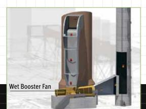
reduced. As a conservative estimate, the energy use of each booster fan, at nominal load and 2.000.000 Nm3/h gas volume, is reduced from 11,6 MW to 9,5 MW.
