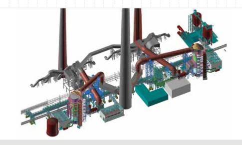
When a power station changes over to non-reheated FGD wet stack operation, it is very important to consider the risk of "spitting", which is the emission of droplets of acidic condensate from the top of the chimney. This risk, and possible remedies, can be investigated through a Wet Stack Design Study, which models the behavior of droplets in the outlet ducts and chimney downstream of the FGD system.
