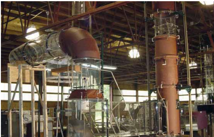
Scale model of ductwork used by Alden Research Laboratory
