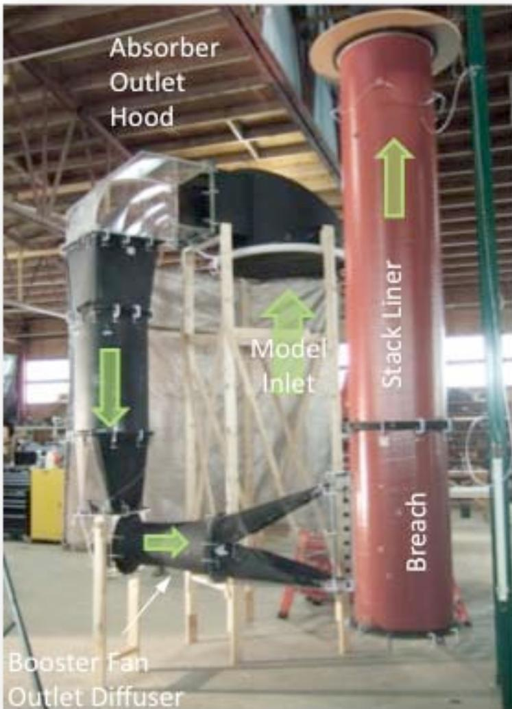
*Figure 4: Detailed scale model of the FGD plant, outlet duct and chimney breaching to develop, test and validate the proposed liquid collector and drain system.*
