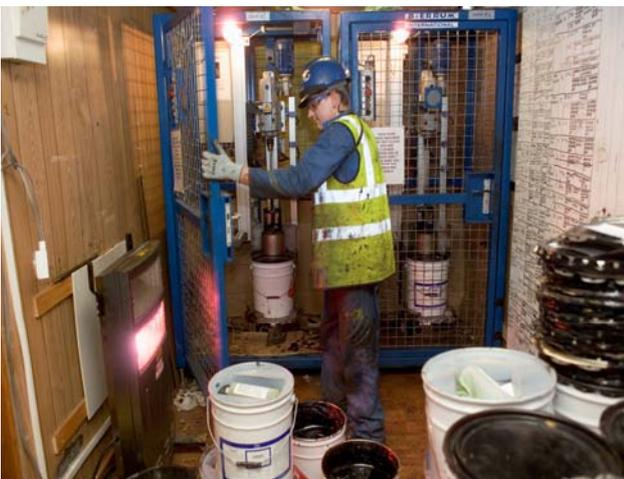
Figure 14: Machines for mixing the Pennguard® Adhesive Membrane
