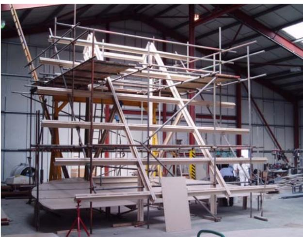
Figure 8: Trial erection of the GRP at the factory
