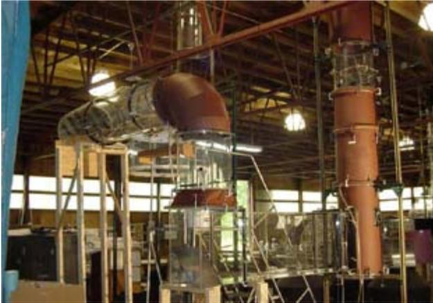
**Figure 3: 1/16 scale model of ductwork used by Alden Research Laboratory**
